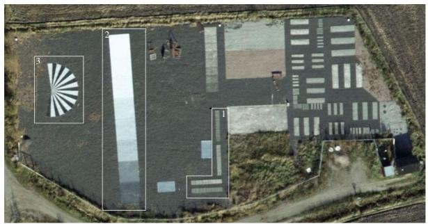
Figure 1. Overview of Sjökulla test site during testflights. The test figures used in this studyare: 1) permanent dense spatial resolution test bar targets, 2) transportable grey scale with 8 steps and 3) transportable Siemens star. Photo by Meixner.
